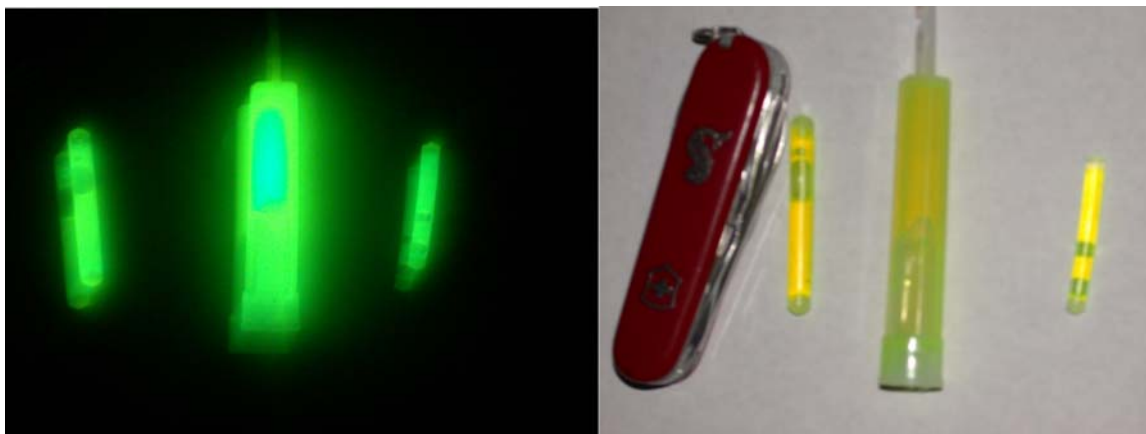
Figure 1. Green (Cyalume Lightsticks™) chemical lightsticks (5.1 cm, 10.2 cm, and 3.8 cm from left to right) used in feasibility testing at Bonneville and McNary Dams and in evaluation of camera tracking arrays. (Studies conducted by PNNL for Portland and Walla Walla District USACE, respectively.)
