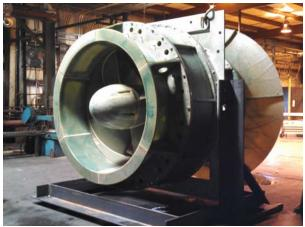
Source: Amjet Figure 1-9. Composite housing with combined turbine/ generator assembly
