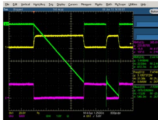
SiC module under electrical testing SiC module Switching Waveforms
