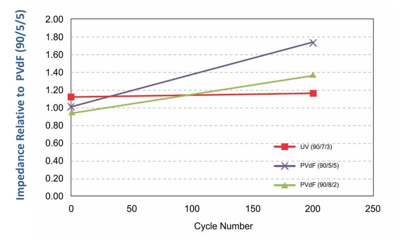
Pouch Cell AC Impedance @-10°C 5.8 mg/cm2, 25 µm thick, NMC 111, carbon, UV binder
