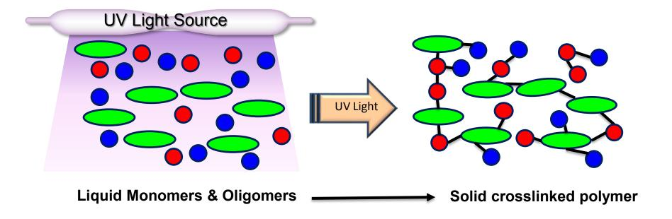
UV Light instantly polymerizes photoreactive mixture into a solid plastic.
