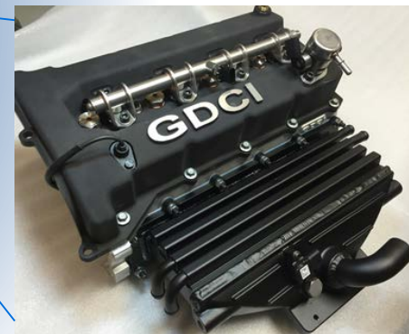
Cylinder head with compact, integral exhaust manifold with pre-turbo catalyst
