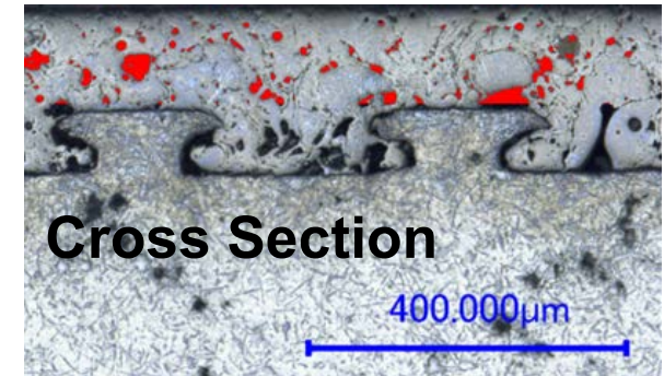
PTWA Coating with 6-8% Porosity
