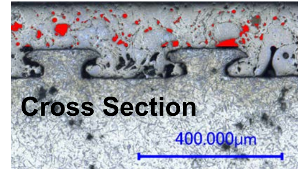
PTWA Coating with 6-8% Porosity
