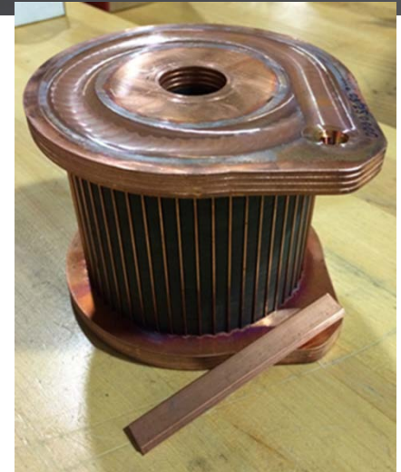
Rotor fabricated by Friction Stir Welding
