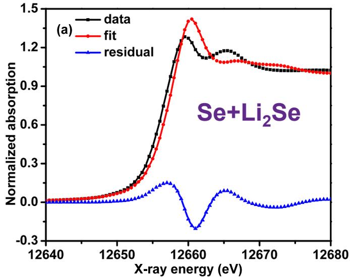
**Se and  $\text{Li}_2\text{Se}$  two phase-transition is impossible.**
