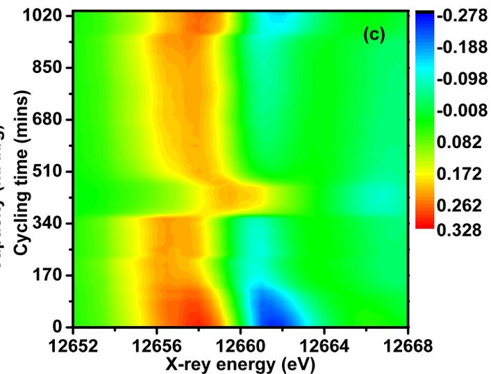
Se K-edge of  $\text{Li}_2\text{Se}$  shifted to high energy may be caused by the strong columbic interaction between  $\text{Se}^{2-}$  and surrounding lithium leading to reduction in the screening effect .
