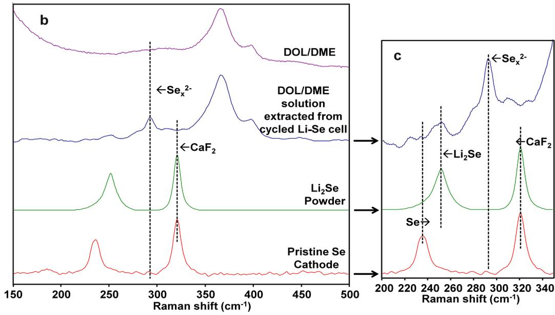
Raman spectroscopy of DOL/DME solvent, the Li-Se cell rinsing solution, Li<sub>2</sub>Se powder and pristine Se cathode for comparison.
