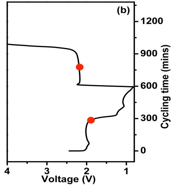
The complete conversion of Se to Li<sub>2</sub>Se by the end of the discharge.
