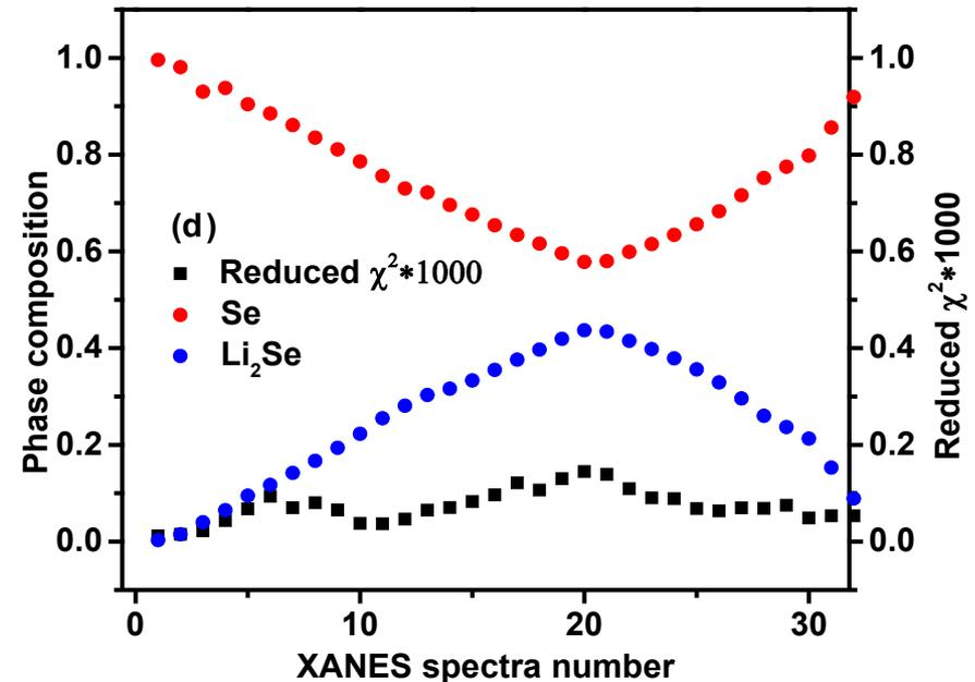
$\text{Li}_2\text{Se}$  is formed and increasing in composition with discharge to 0.8V, then oxidized to Se with charge.
