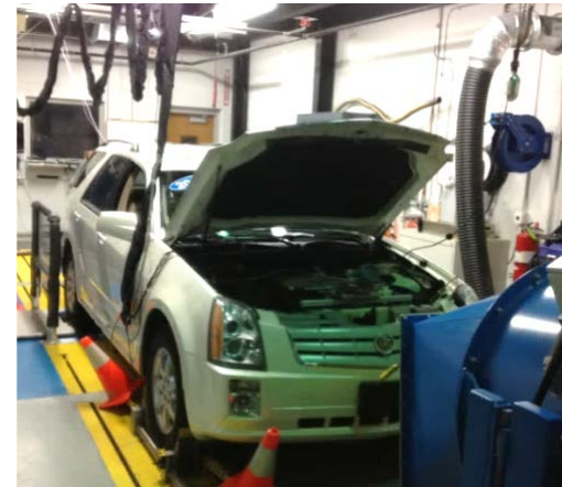
Cadillac SRX has same DOHC V6 engine used in Sequence VID test
