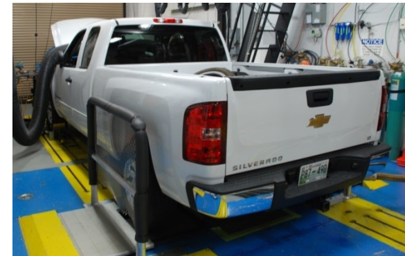
Experiment repeated in vehicle with pushrod V8 engine on 2 lubes (Mobil1 and PNNL prototype)
