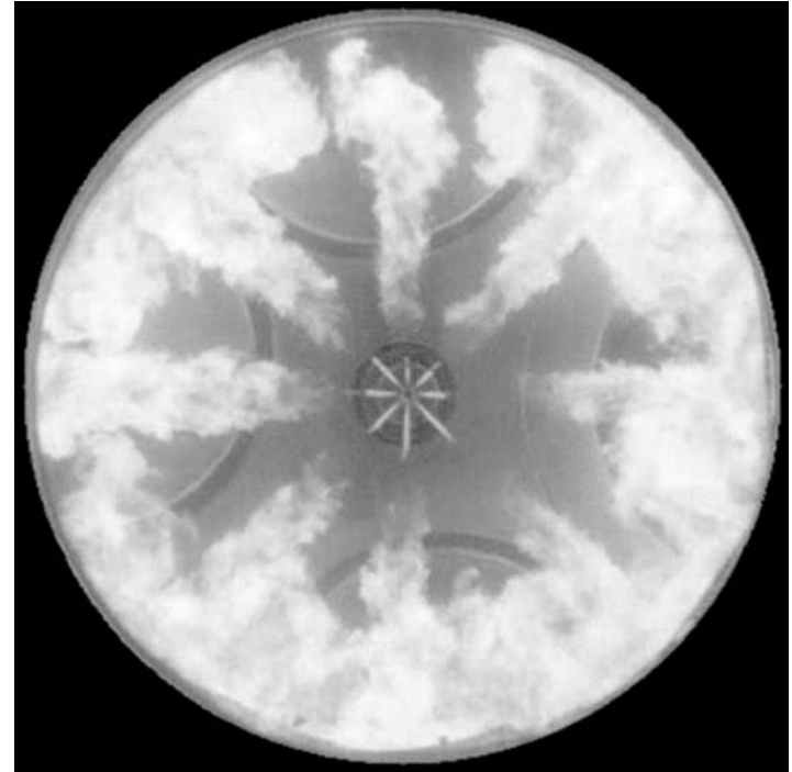
Diesel spray combustion imaging through transparent piston (Mark Musculus, Sandia)
