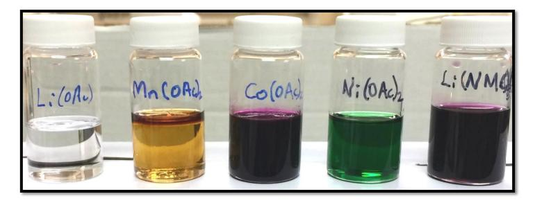
Room temperature DESs of different metals for battery materials. The DESs show clear solutions of the metal acetates dissolved in glycerol (shown are with 1:5 molar ratio).
