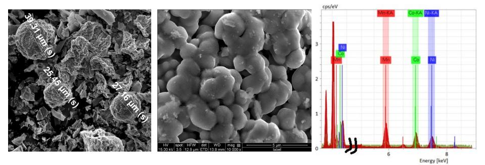
The NMC powders show a wide range of morphologies, including spheres consisting of secondary particles.
