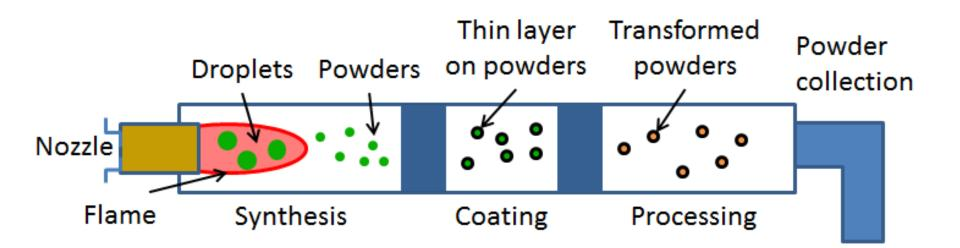
The battery powder production is aimed at integrating synthesis, coating, and processing into one process. The materials produced are ready for use in battery cathode fabrications without further processing.
