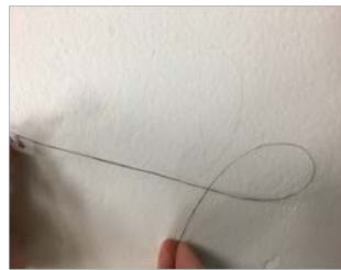
Produced carbon fibers from M4 precursor can be easily wrapped around a core with a diameter of 1"
