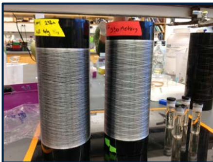
Spools of bacterially produced spider silk protein, 350m of 8-fiber thread.
