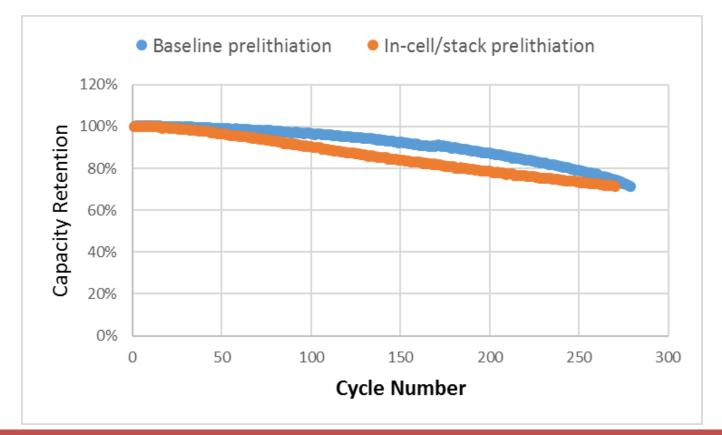
Cycle life can be further improved by optimizing the prelithiation solvent and additive formulation, as well as protocol conditions
