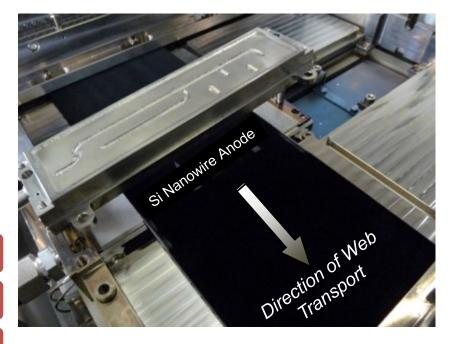
During Q1 2016, Amprius tested a first of its kind pilot line tool for rollto-roll production of double-sided, rooted silicon nanowire anodes Approach:
