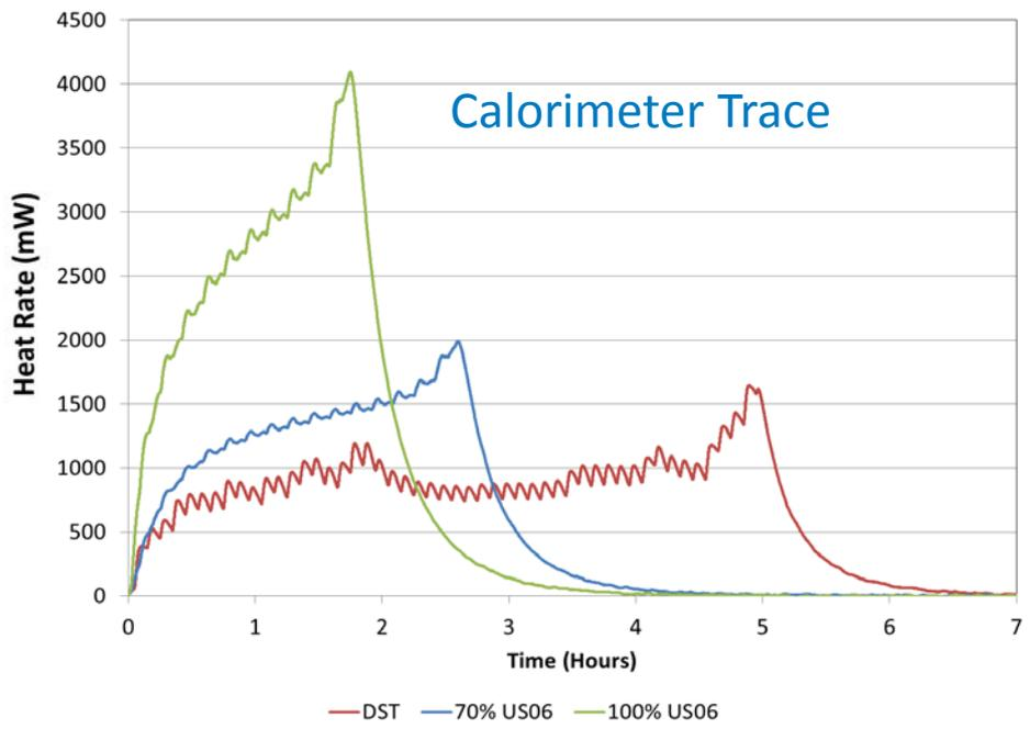
Calorimeter can measure the efficiency and heat generation under various drive cycles—helps in designing thermal management systems for battery packs.
