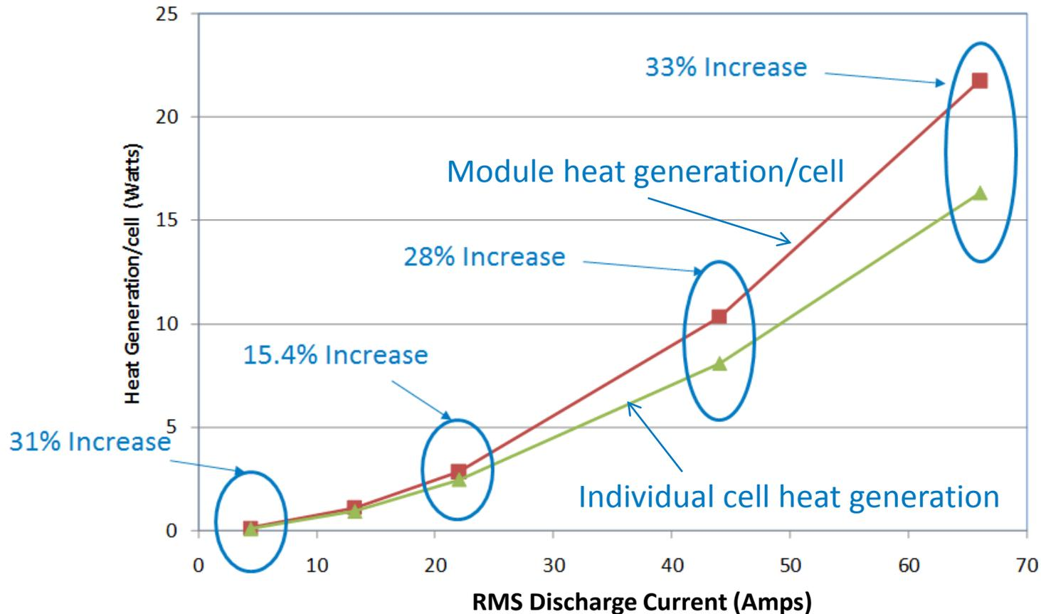
Heat generated by interconnects is important to understand in order to properly design a thermal management system
