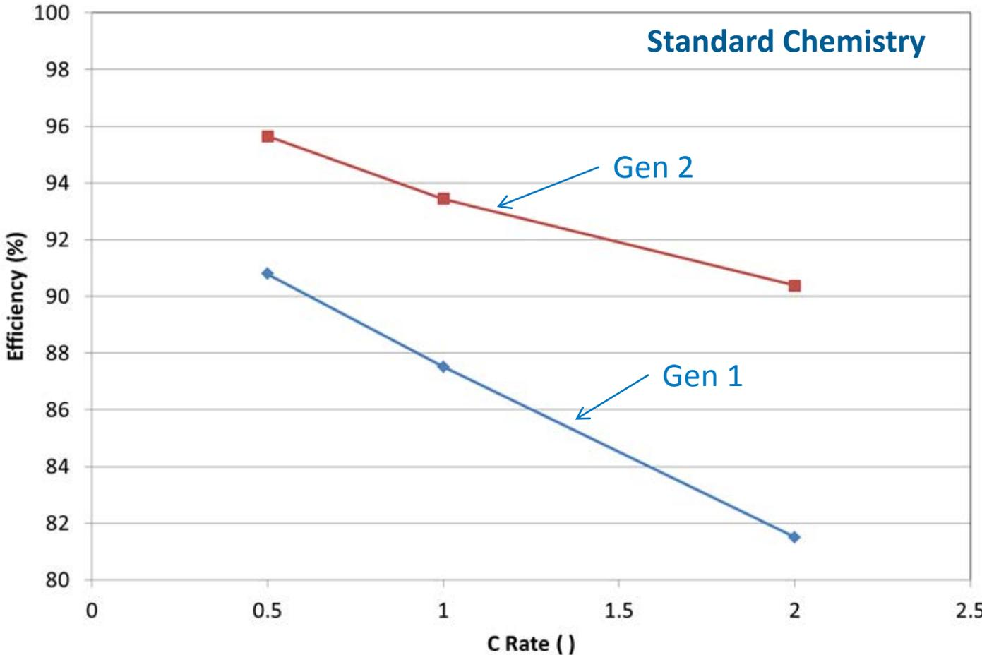
During the USABC programs, electrochemical and mechanical design changes are made to the cells. Calorimetry can determine if the changes are positive.
