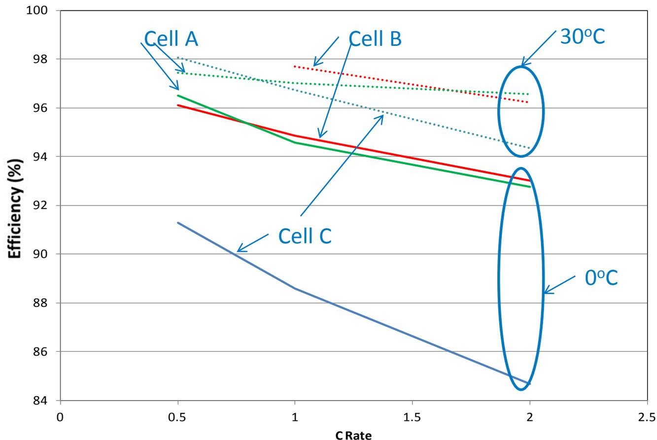
Testing the efficiency of cells at multiple temperatures shows how different additives/designs will affect performance.
