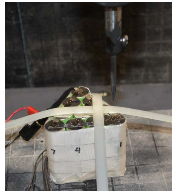
1S10P Battery: Failure point on edge cell
