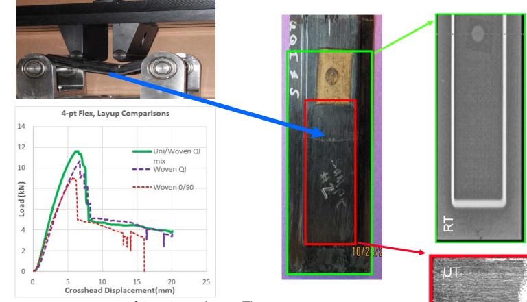
Several types of potential inservice damage were induced on carbon fiber composites Including:
