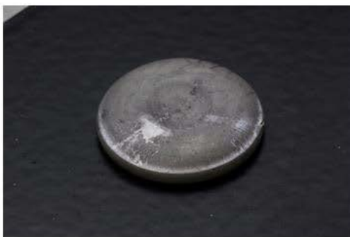
UPJ8-5 2.2 mm (Powdercoated) Al 6013-T4 (Pre-treated) AM60
