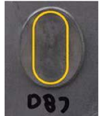
Experimental Oval Boss Head Shape with Hole Shape Superimposed
