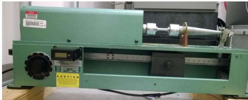
Rotary Beam Fatigue testing machine creates simple completely reversed stress cycle R=-1 . Tests conducted at 10,000 RPM
