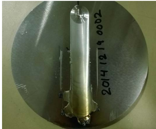
Bead on plate processed region on a plate cut from the forged billet
