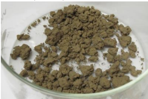
Nanoamor's 50 nm silicon coated with 10% w/w PFM (before milling)
