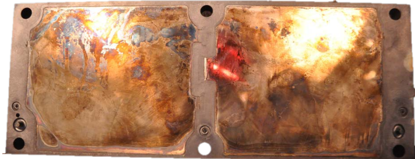
Bottom - electrically active (color due to soaking module to dissolve potting material)
