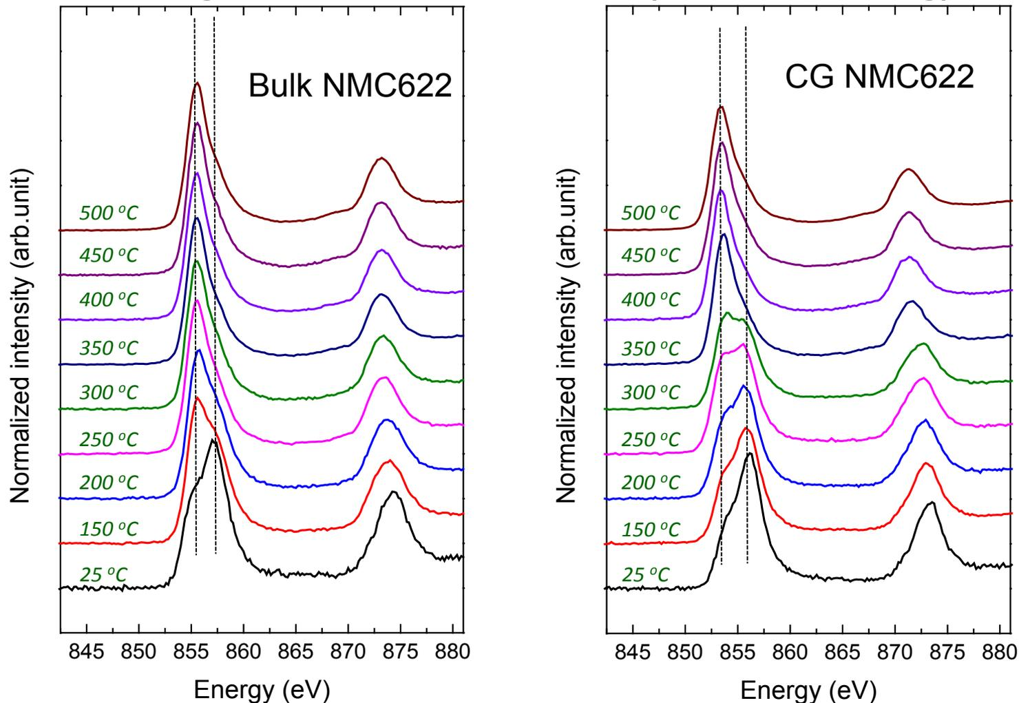
Ni reduction reflected as the lower energy peak occurred quickly at low temperature (~150 °C) in bulk NMC622. In contrast, CG NMC622 is more stable and Ni is stable up to 250 °C and gradually reduced, and completed at 350 °C
