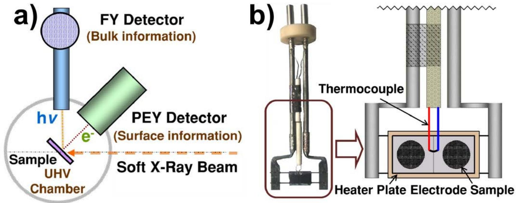
The partial electron yield (PEY) measurement in soft XAS gives information about surface properties (up to  $\sim 5$  nm), while the fluorescence yield (FY) measurements probes bulk properties (up to  $\sim 300$  nm).
