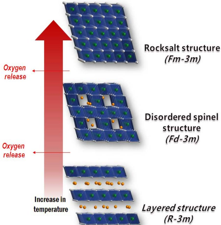
Typical phase transition of Ni-based layered cathode materials during thermal decomposition by heating
