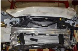
Extruded Aluminum Front Bumper and Crush Can
