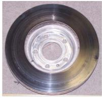
(b) Coated Rotor After Test
