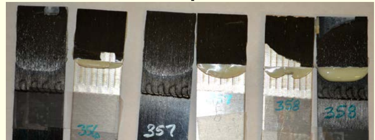
Laser-structured joints: 460 - adhesive
