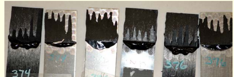
Laser-structured joints: 620 adhesive
