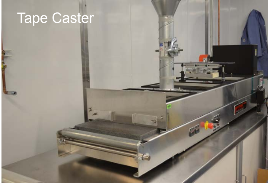
9 Heating Zones -2 IR Lamps -7 Convective Air Zones
