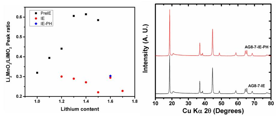
• Post heated sample does not show any significant structural changes
