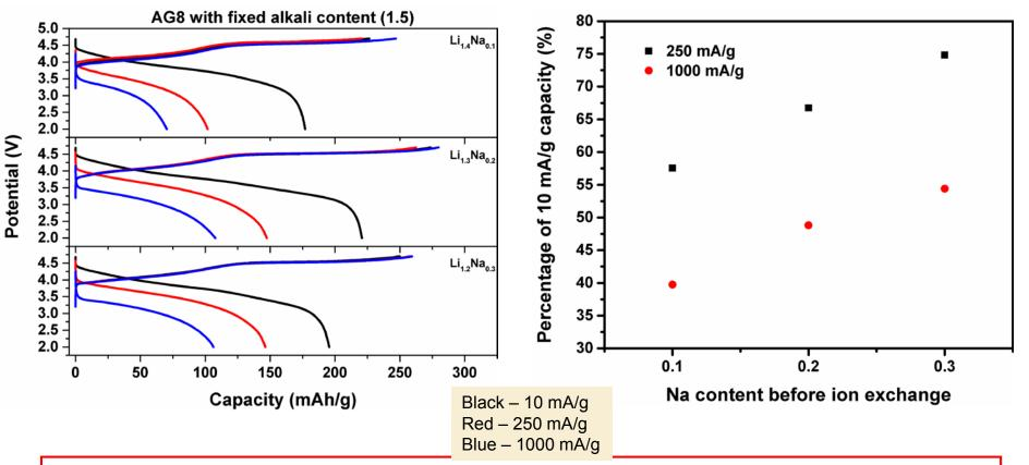
Rate capability of samples is improved when the starting material has more sodium content
