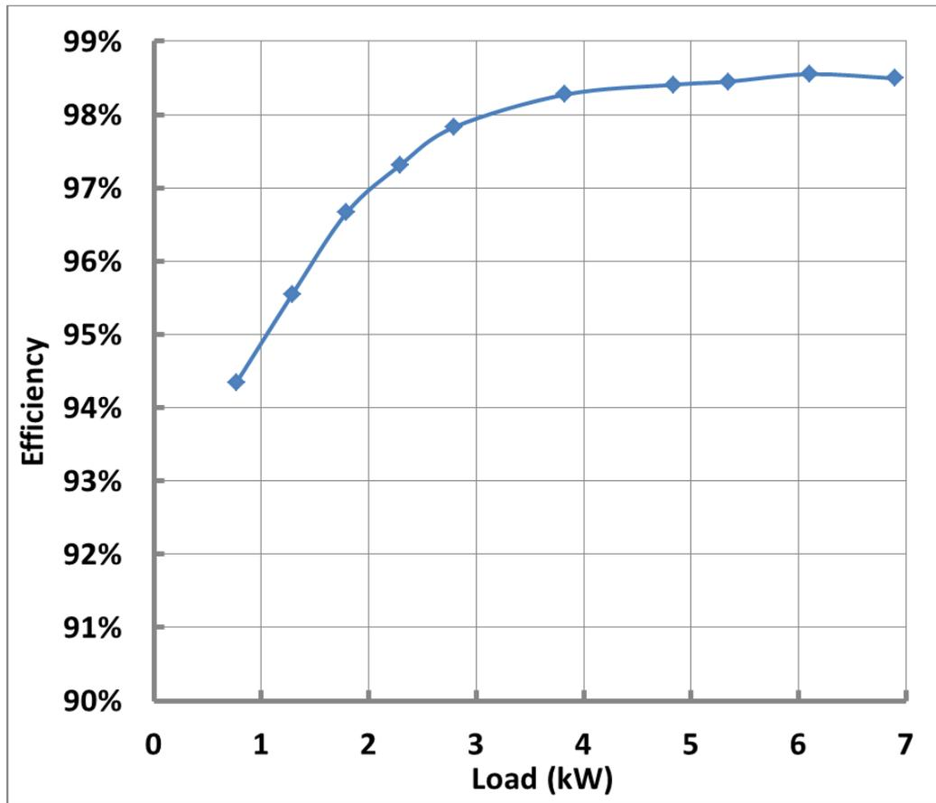
**Charger front end converter efficiency v.s. output power**
