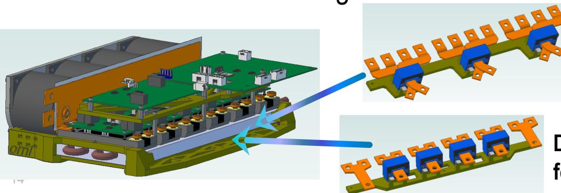
Segmented 3-phase inverter for single motor systems
