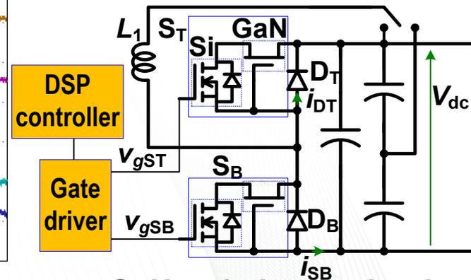
GaN switch test circuit
