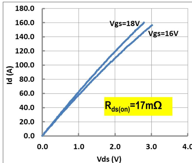
SiC MOSFET phase-leg modules static characteristics
