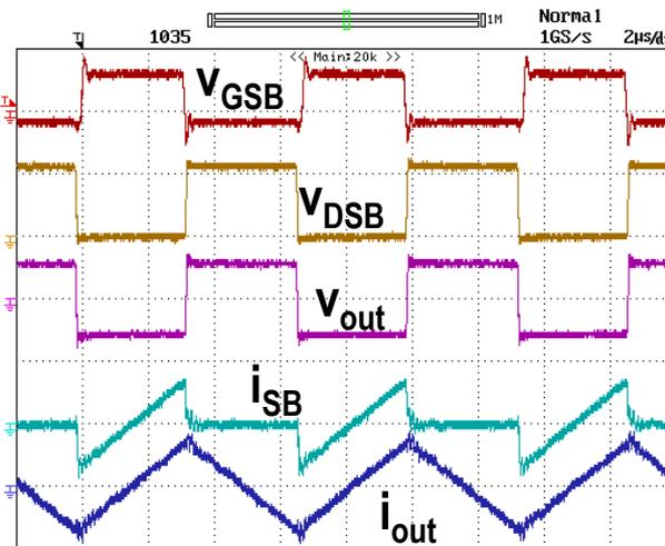
$V_{GSB}$ , 20V/div;  $V_{DSB}$ ,  $V_{out}$ , 300V/div;
