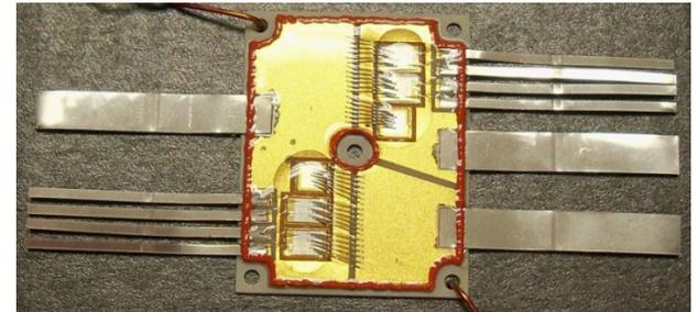
SiC MOSFET phase-leg modules (36x46mm): 1200V/100A
