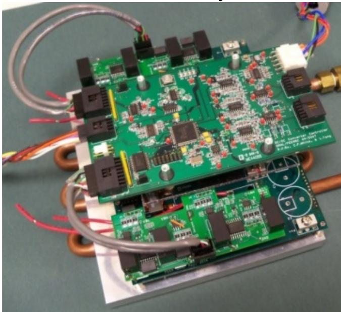
3-port 6.6 kW SiC bidirectional isolation converter
