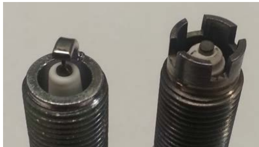
Conventional Spark Plug (0.7mm gap axial direction)
