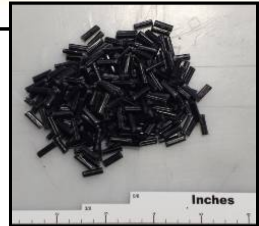
0.43" long glass fiber (50 wt%)/PA66 pellets
