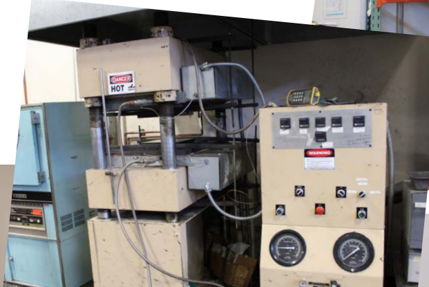
Hydraulic compression Press 150 ton 750F capable
