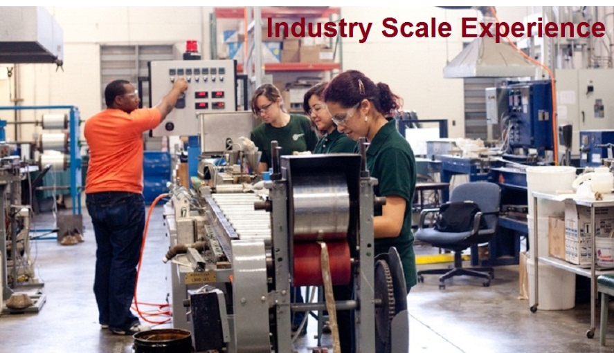
Theresa Bayush (MS candidate) and Melike Onat (PhD candidate) working on natural fiber extrusion
