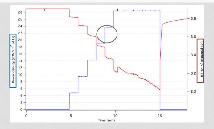
Lithium–LiCoO<sub>2</sub> experiment: Discharge rate and power of about 10 mA/cm<sup>2</sup> and 30  $mW/cm^2$  of anode rod was possible even though the distance between the rod and plates can be as high as 1 mm. Note: other 3d batteries: 1 mW/cm<sup>2</sup>, not scalable, only nano.
