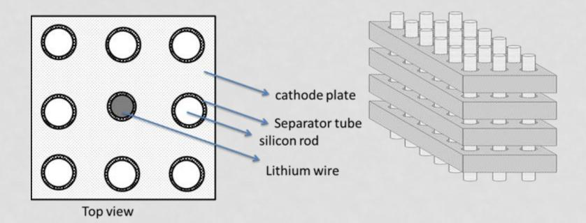
The presence of auxiliary lithium rods can compensate for the lithium-ion loss.
