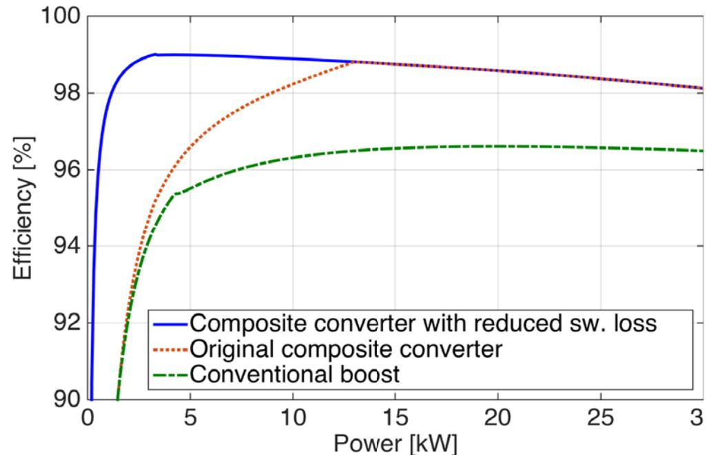
Comparison of efficiency curves at  $V_{batt} = 250\text{ V}$ ,  $V_{bus} = 650\text{ V}$
