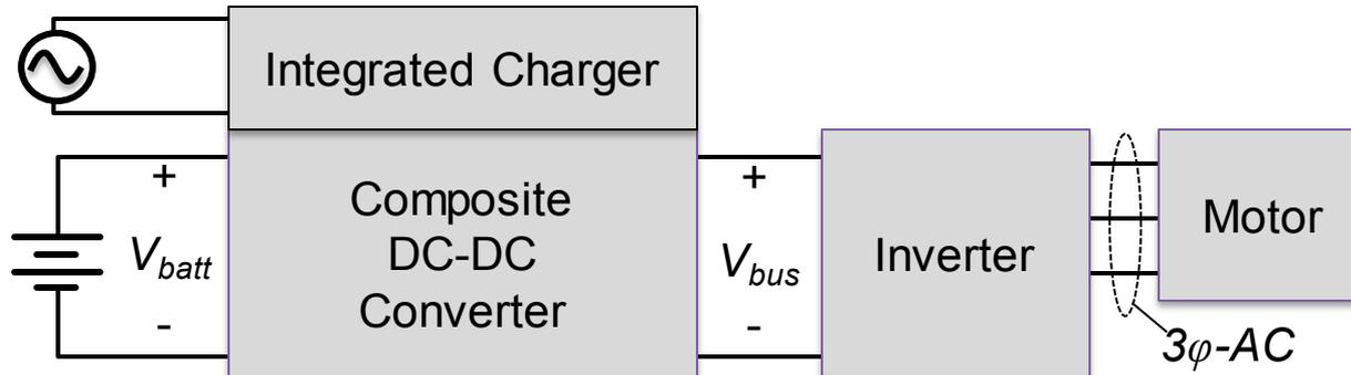
Demonstrate new composite converter topology that leads to fundamental performance improvements including average efficiency, film capacitor size, and on-board charger size.
