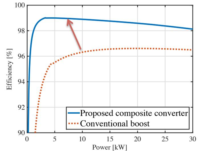
Efficiency improvement in proposed composite architecture vs. conventional boost:  $V_{batt} = 250 \text{ V}$ ,  $V_{bus} = 650 \text{ V}$
