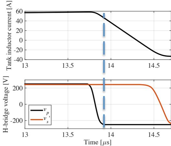
At light load, tank inductor does not have enough energy to achieve primary side full ZVS. Active switching causes switching loss
