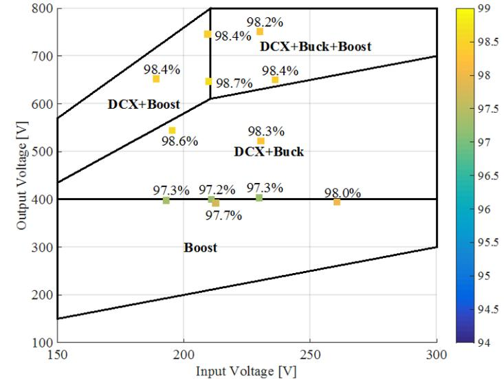
Comparison of predicted efficiency characteristics using detailed loss model calibrated to experiment
