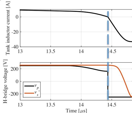
Use of magnetizing current to assist ZVS at low power, plus additional commutation (dead) time, extends ZVS range
