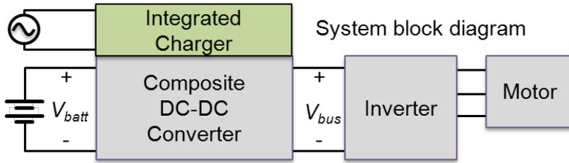
Selected system architecture: charger integration within the composite DC=DC converter
