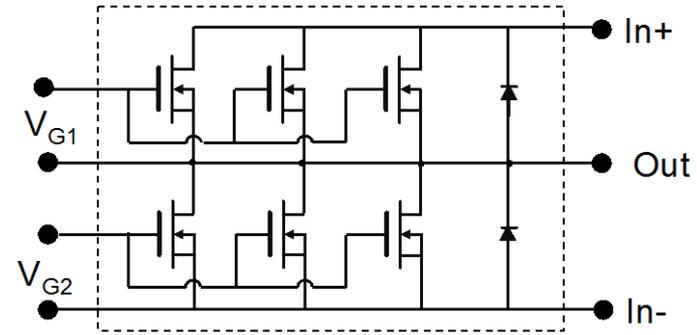
Half-bridge SiC MOSFET module to be packaged for 20 kW demonstration
