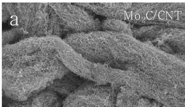
SEM images of Mo<sub>2</sub>C/carbon nanotubes
