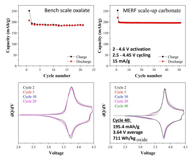
Voltage fade is almost entirely suppressed in scaled up electrode, if capacity is restricted to ~200 mAh/g
