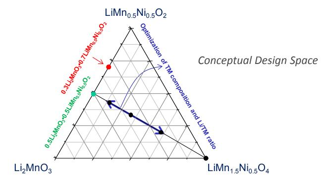
Electrodes on 'layered-layered-spinel' tie-lines have a constant Mn:Ni ratio, e.g., 3:1 on the 0.5Li<sub>2</sub>MnO<sub>3</sub>•0.5LiMn<sub>0.5</sub>Ni<sub>0.5</sub>O<sub>2</sub> - LiMn<sub>1.5</sub>Ni<sub>0.5</sub>O<sub>4</sub> line
