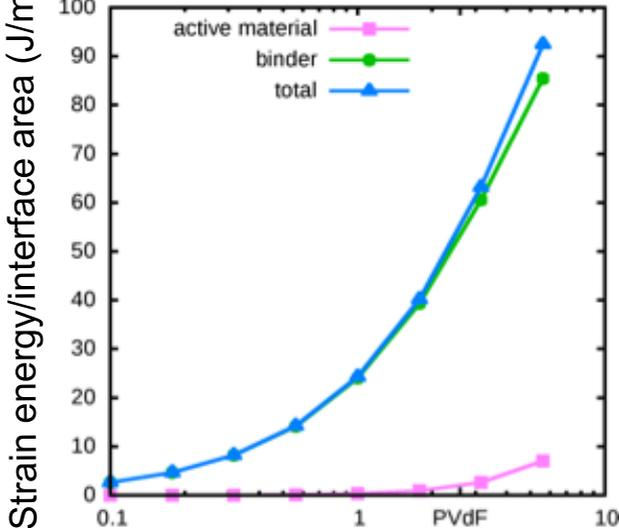
Model allows exploration of impact of size, binder properties, and binder-Si adhesion energy on cracking and de-lamination
