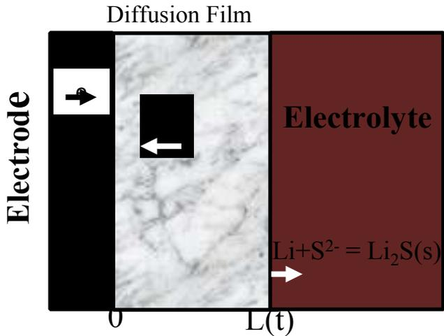
$$\frac{\partial C_i}{\partial t} = D_{eff} \left( \frac{\partial^2 C_i}{\partial x^2} \right)$$
