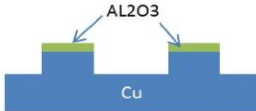
Configuration to measure SEI growth on Cu
