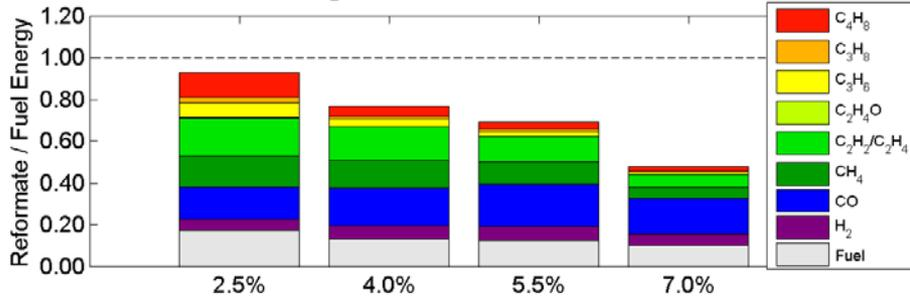
IsoOctane NVO Fuel Injection Sweep (SOI: 40 deg bTDC; O<sub>2</sub>: 4%)
