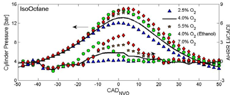
Ethanol NVO Fuel Injection Sweep (SOI: 40 deg bTDC; O<sub>2</sub>: 4%)
