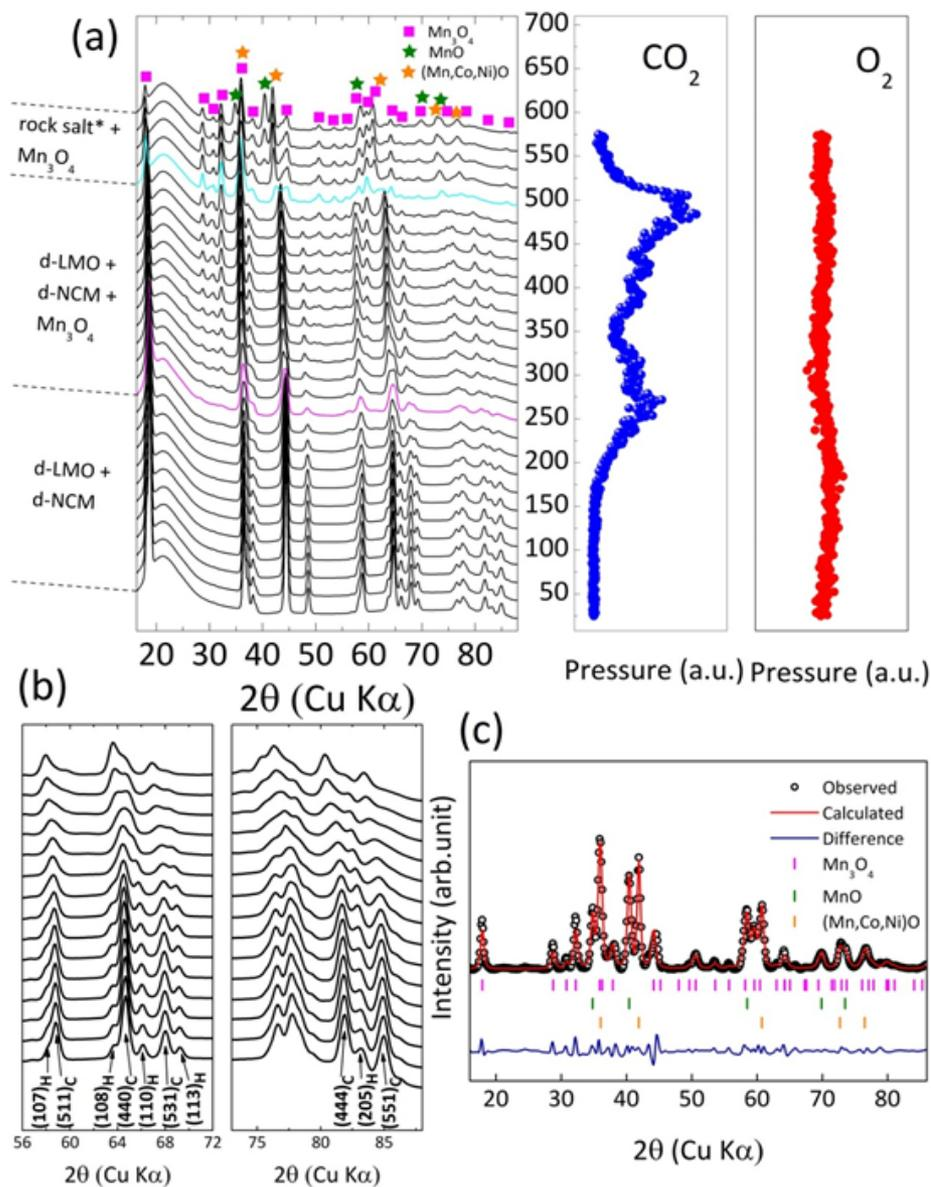
(a) *In situ* XRD-MS data of electrochemically delithiated LMO and NCM mixture with weight ratio of 3:1, and (b) zoomed in XRD patterns with  $(hkl)_H$  and  $(hkl)_C$  indexed for hexagonal NCM and cubic LMO respectively; patterns are only shown up to  $300^\circ\text{C}$  for clarity. (c) LeBail fitting of the XRD pattern at  $580^\circ\text{C}$ . \*rock salt phases include  $\text{MnO}$  and  $(\text{Mn,Co,Ni})\text{O}$ ; their forming temperatures are close to each other.
