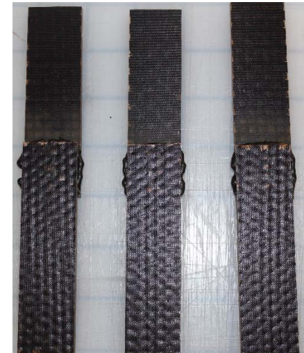
(b) Bonded joints with Active Adhesive for DIS-ASSEMBLY
