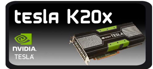
Majority of Titan's speed comes from NVIDIA K20 GPUs
