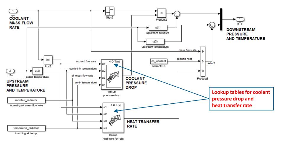
Top-level of the demonstration model in Simulink
