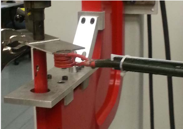
Induction heat station integrated to SPR unit.
