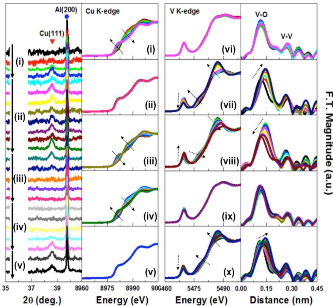
Complete information on structural/chemical evolution of  $\epsilon$ -CVO with cycling was obtained *via* simultaneous *in-situ* XRD/XAS, indicating:
