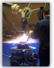
Aluminum brake rotor with thermally sprayed wear resistant coating
