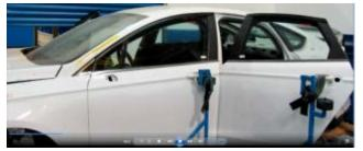
Side Door Glass - Door Slam Durability Test
