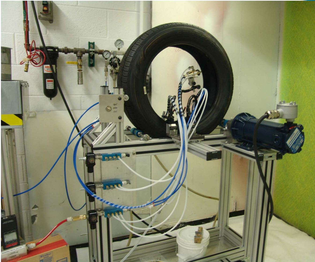
Tire Rotated, Stationary Spray Heads
