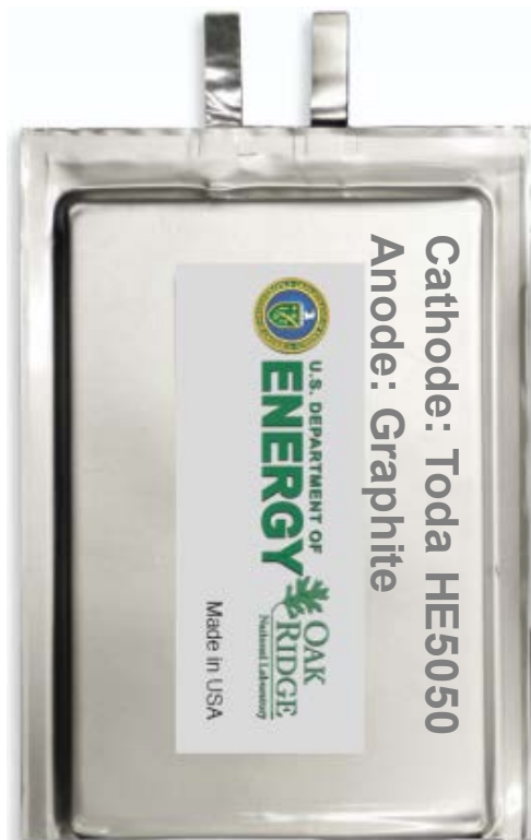
Pouch cell with 3 unit cells
