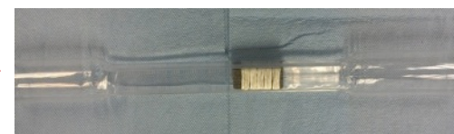
Catalyst loaded into quartz tube reactor
