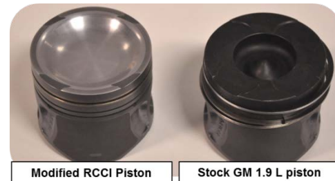
RCCI Piston designed for premixed LTC
