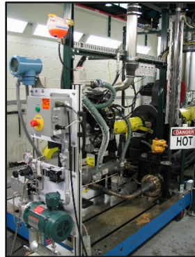
SIDI gasoline: Opel 2.2 L Ecotec engine Test data. Vehicle: Conventional midsize, different Powertrain assumptions from HCCI
