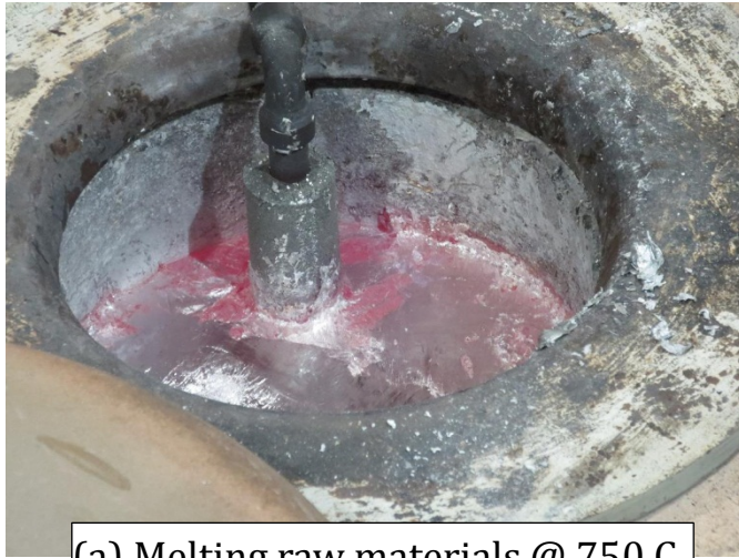
(a) Melting raw materials @ 750 C.
