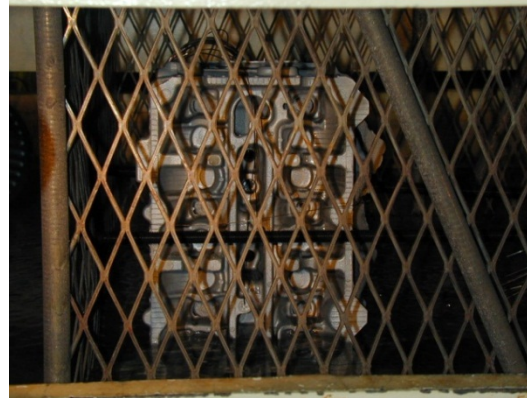
Drop bottom HT furnace and Quenching basket
