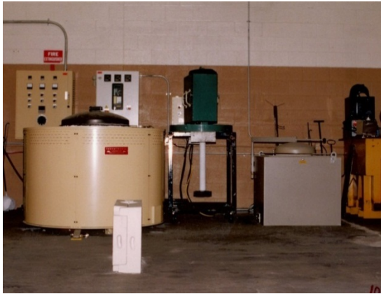
Electric melting furnaces and flux unit Sand mixer and sand mold
