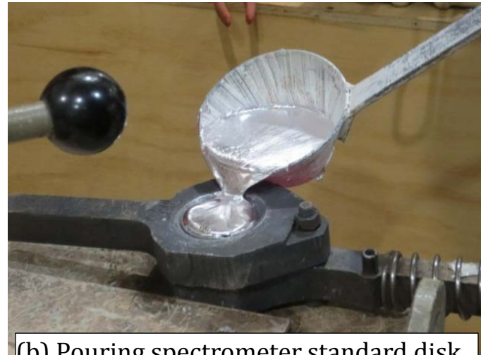
(b) Pouring spectrometer standard disk to control melt composition.
