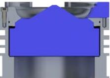
(SNL) Completed design of contoured bowl for multiple injections coupling with bowl shape, install late FY14
